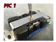
**Step 1.** Remove the center screw from the back of the outlet.
