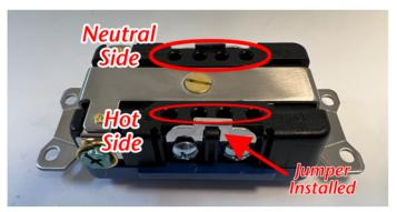
With the jumpers removed, the pairs of holes closest to each clamp screw are still connected, but the pairs are independent of each other.
