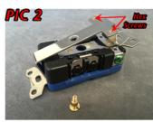
**Step 2.** Pry the mounting bracket off of the outlet.
