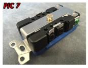
**Step 6.** Reassemble the 4181US, ensuring that the gasket stays in place while you snap the mounting bracket back on, and replace the center screw.
